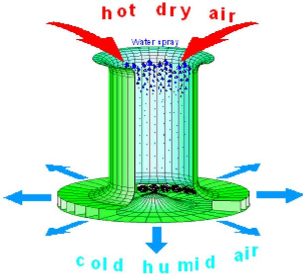
Fig. 1. ET principle of operation.
