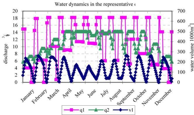
Fig. 6. Discharges of  $q_1$  (from the sea to the lower reservoir), water volume in the lower reservoir  $v_1$ , and  $q_2$  (spraying discharge) during the representative days. Each month is represented by 24 h.
