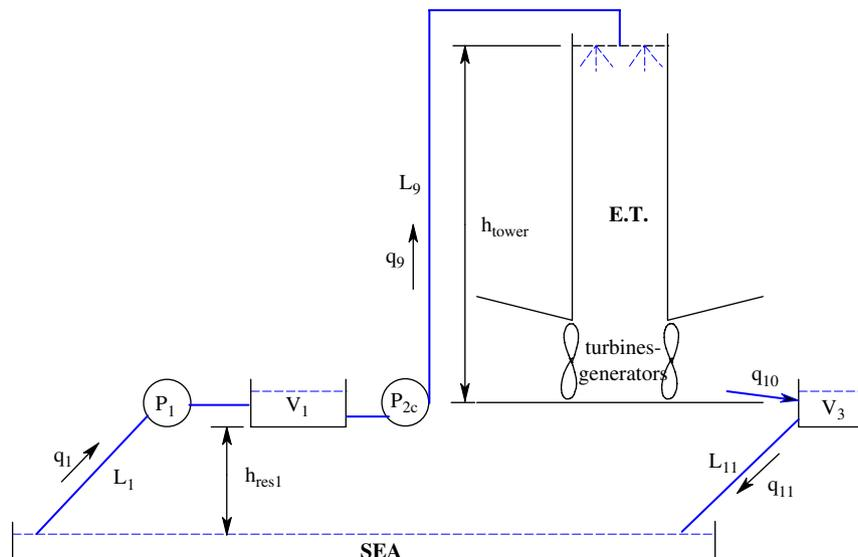
Fig. 2. A scheme of the stand-alone ET.
