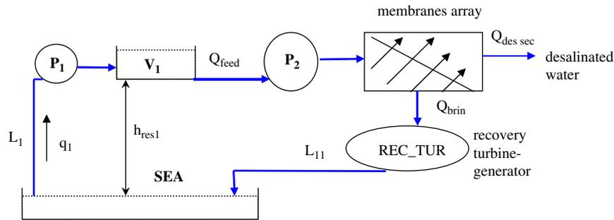
Fig. 4. A scheme of the stand-alone seawater desalination plant.
