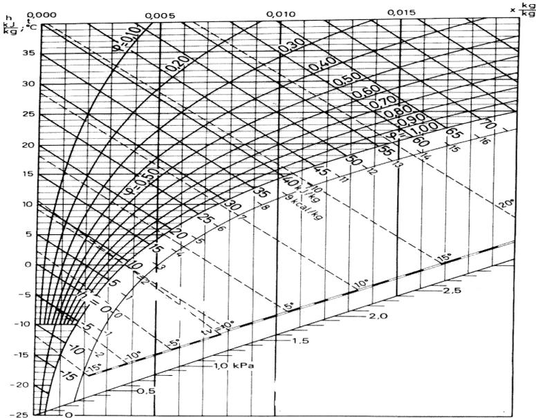
Based with an ambient air temperature of 15°C and relative humidity of 40% across the tower height of 100m to lower the temperature of 3000m<sup>3</sup>/s of air requires removal of 15° X 3000m<sup>3</sup> X 1.186 kg/m<sup>3</sup> with air having a specific heat of 1.012 J per g per K or 1012 J per Kg per K
