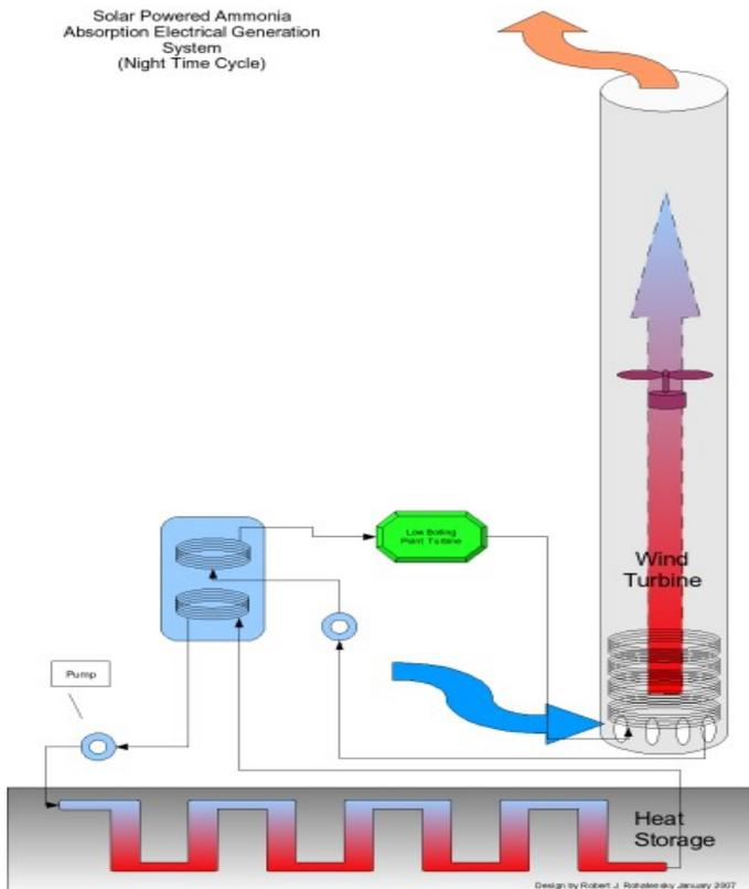
Depending on the design of the thermal storage there will be losses with heat dissipating into the earth, as an estimate 50% of the stored heat can be used at night. The intent of the night system is to generate some power while “cooling off” the thermal storage.
