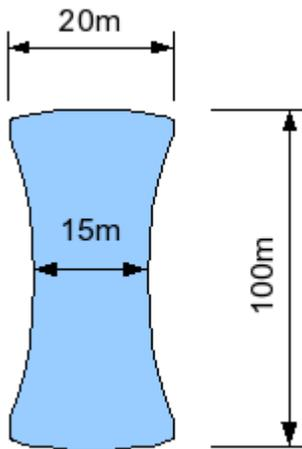
Assuming a medium scale system with a tower height of 100m and a diameter of 20m narrowing to 15m in the center. The tower will function bi-directionally seasonally and the wind turbine would be located at the center of the tower with a diameter of 15m.
