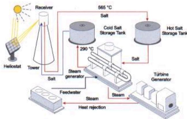
Figure 3.3 Overview of a Power Tower system (SunLab, 2001)
