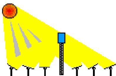
Figure 4.1 *Principle of a Power Tower (SunLab, 2001)*
