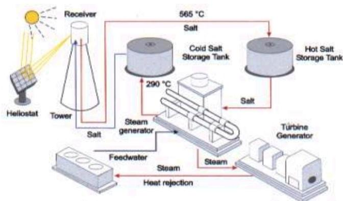
Figure 4.2 A schematic Power Tower system (SunLab, 2001)
