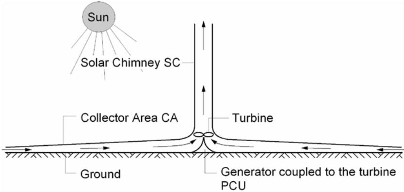
FIGURE 3 - SCHEMATIC WORKING PRINCIPLE OF A SCPP
