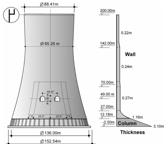
FIGURE 1 - COMPONENTS AND DIMENSIONS OF THE 200M NDCT AT NIEDERAUSSEM POWER STATION
