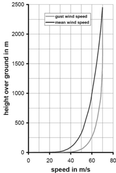
FIGURE 7 – PROFILES OF MEAN AND GUST WIND SPEED
