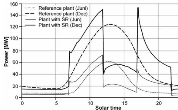
FIGURE 6 - PEAK-LOAD SERVICE OF A SCPP WITH DOUBLE GLAZED CA
