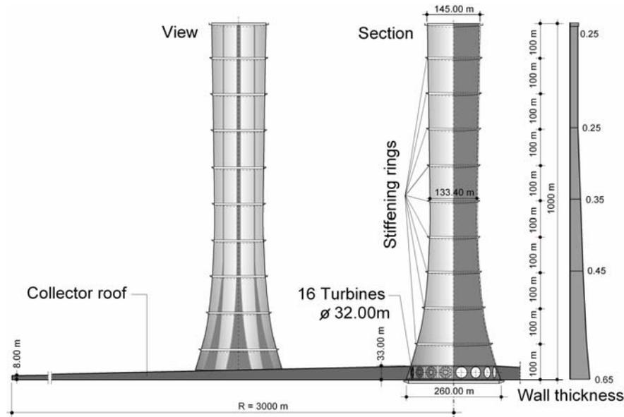
FIGURE 2 - 1000 M CHIMNEY FOR A 200 MWP SCPP
