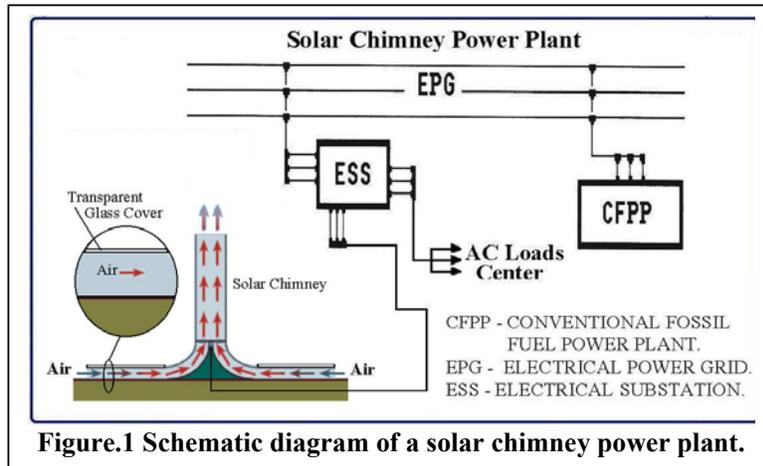
Figure.1 Schematic diagram of a solar chimney power plant.
