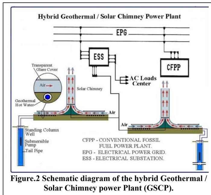
Figure.2 Schematic diagram of the hybrid Geothermal / Solar Chimney power Plant (GSCP).
