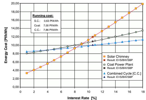
Fig. 12. Energy production costs from solar chimneys, coal and combined cycle power plants depending on the interest rate.
