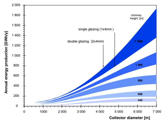
Fig. 3. Annual energy production by a Solar Chimney (at 2300kwh/m<sup>2</sup>/a global insolation) dependent on collector diameter and chimney height.
