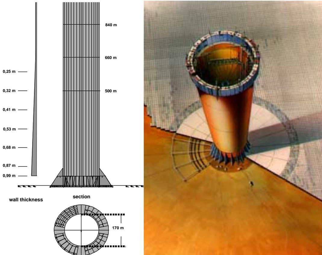
Fig. 11. Wall thickness of a chimney tube 1,000 m high and 170 m in diameter and artist view of a 1,000 m chimney tube under construction.
